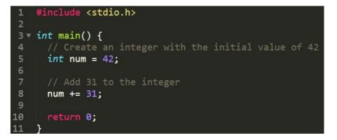
We can compile C programs using gcc to generate a binary executable
