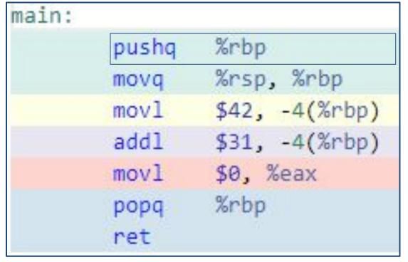
First, we **push** the **base pointer** (%**rbp**) onto the stack for later
