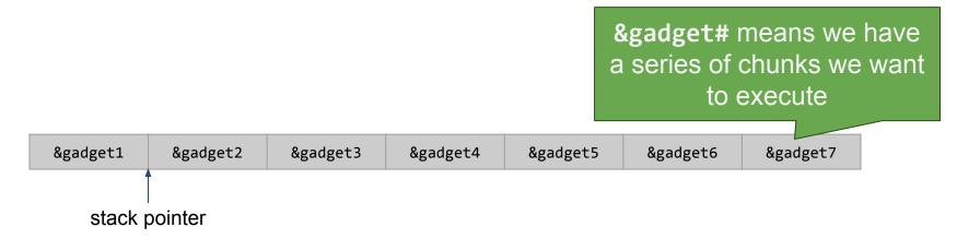
The stack pointer (%esp) is pointing to the location that the CPU is going to fetch instructions and execute them
